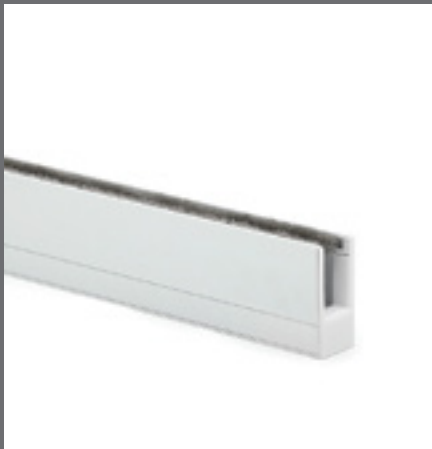
Side channels with light blocking brushes prevent light leakage at the sides of shades for total blackout. (available in white, bronze, black, and clear anodized)
